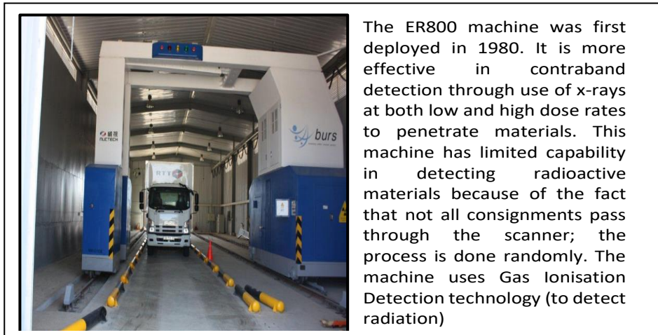
Figure 7: BURS Cargo Scanner with Radiation Portal Monitor
